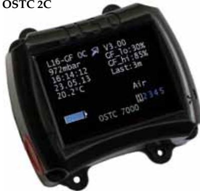
As a user of the 2 since I dive tested the development and Beta test models, I love the screen and the easy menu system. The 2C is bigger (80 mm x 68 mm x 34 mm) and has a 2.4" TFT IPS LCD screen for crystal clear viewing. Unlike the OLED display, the black is now a 'turned on' black pixel, not a blank switched off pixel. A small detail, but it creates a perfect optical display.
